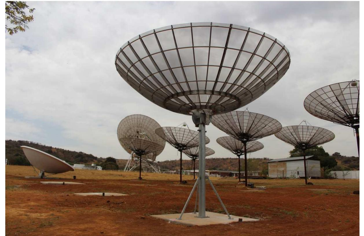
*Fig 2. The 10-dish HIRAX prototype array in the foreground featuring the newly installed NJV Consulting/Rebcon dish at front and centre. The 26m dish at the SAAO Hartebeesthoek site is visible in the background.*
