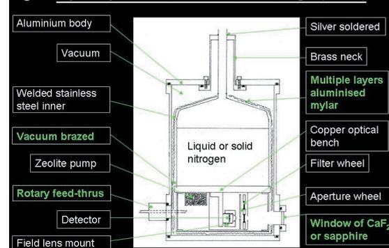
The Dewar I designed could hold liquid nitrogen for about 36 hours and so needed filling only once each day. The first one was in service for about 35 years and is now in the Astronomical Museum at SAAO. Another one is still in active use at Sutherland! Fig. 3 shows how the Dewar was mounted on a telescope as part of a photometer.
