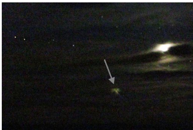
Fig. 3: A single 15 second exposure shows the fuel dump as a bright 1 degree blob (arrowed), easily visible, even with the crescent Moon close by and through thin cloud. This picture was taken at about 03:50 SAST when the 2 nd stage was only at elevation 3.7 degrees and 16 700 km range. At 16 700 km radius, one degree is about 290 km, giving an idea of the actual size of the fuel cloud.
