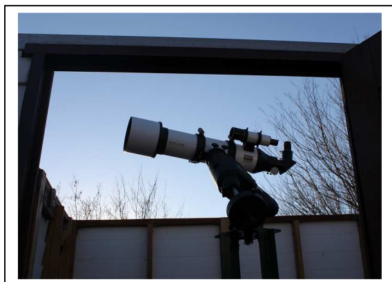
(left) Fig 1. Orion 80mm apochromatic refractor. (right) Fig 2. Refurbished observatory.
