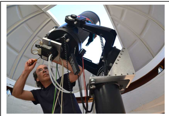
(left, above) Fig 1. Fine-tuning the 300mm Cassegrain. (right, above) Fig 2. The home-made 2m dome.
