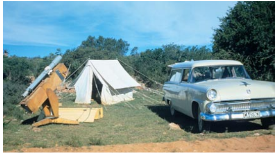
Fig. 5: This picture shows the observing post on the Rooiberg hill near Cillittdorp in the southern Karroo, with a Danjon telescope equipped with a Walraven refractor-photometer. The car is one of the two Ford Range Wagons used by the parties. The picture was taken by one of the principal participants of these site tests, J Dommanget. Credit: ESO, J Dommanget
