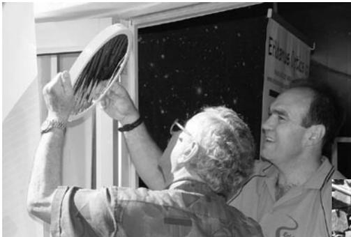
(left) A typical mylar solar filter, here being inspected for pinholes by Jabie Bruwer and Andrie van der Linde. Ensure that the filter fits snugly over the aperture of your telescope so that there is no chance of it being blown off by the wind and causing serious eye damage.
