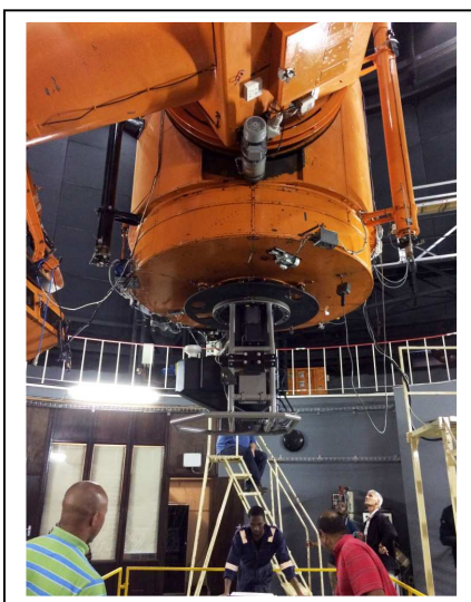
Fig. 3 The upgraded Cassegrain Spectrograph (SpUpNIC) being installed on the 74-inch on 21 October 2015
