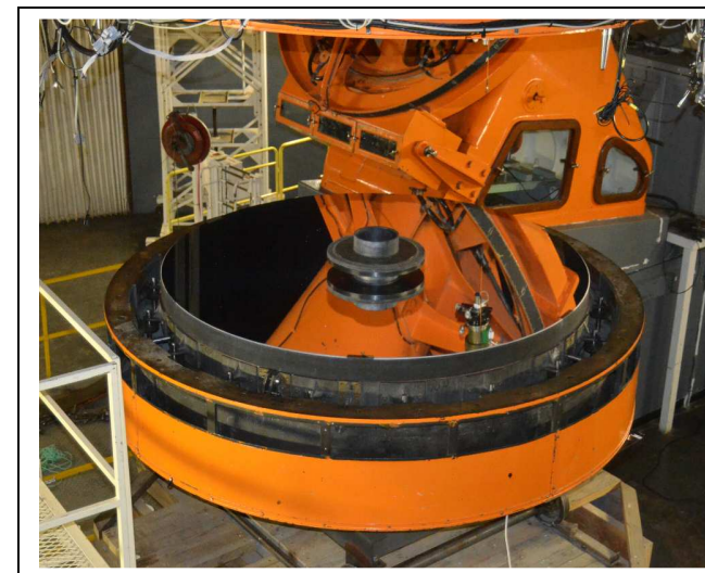
Fig. 7 Re-installing the freshly-aluminised 74-inch primary mirror on 27 November 2015
