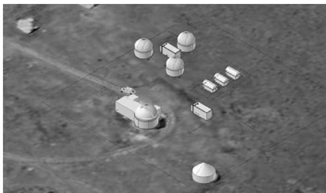
The planned site layout in Sutherland. In the foreground are two existing buildings (a storage rondawel and the IRSF dome) behind which the site will be laid out. Although three buildings of each type are shown here, only two domes and two aqawan enclosures will initially be erected. In 2013 the three best sites in the network will each get an additional 1.0m telescope. The two shipping containers are a site services building (SSB) and storeroom respectively. (Source: LCOGT)
