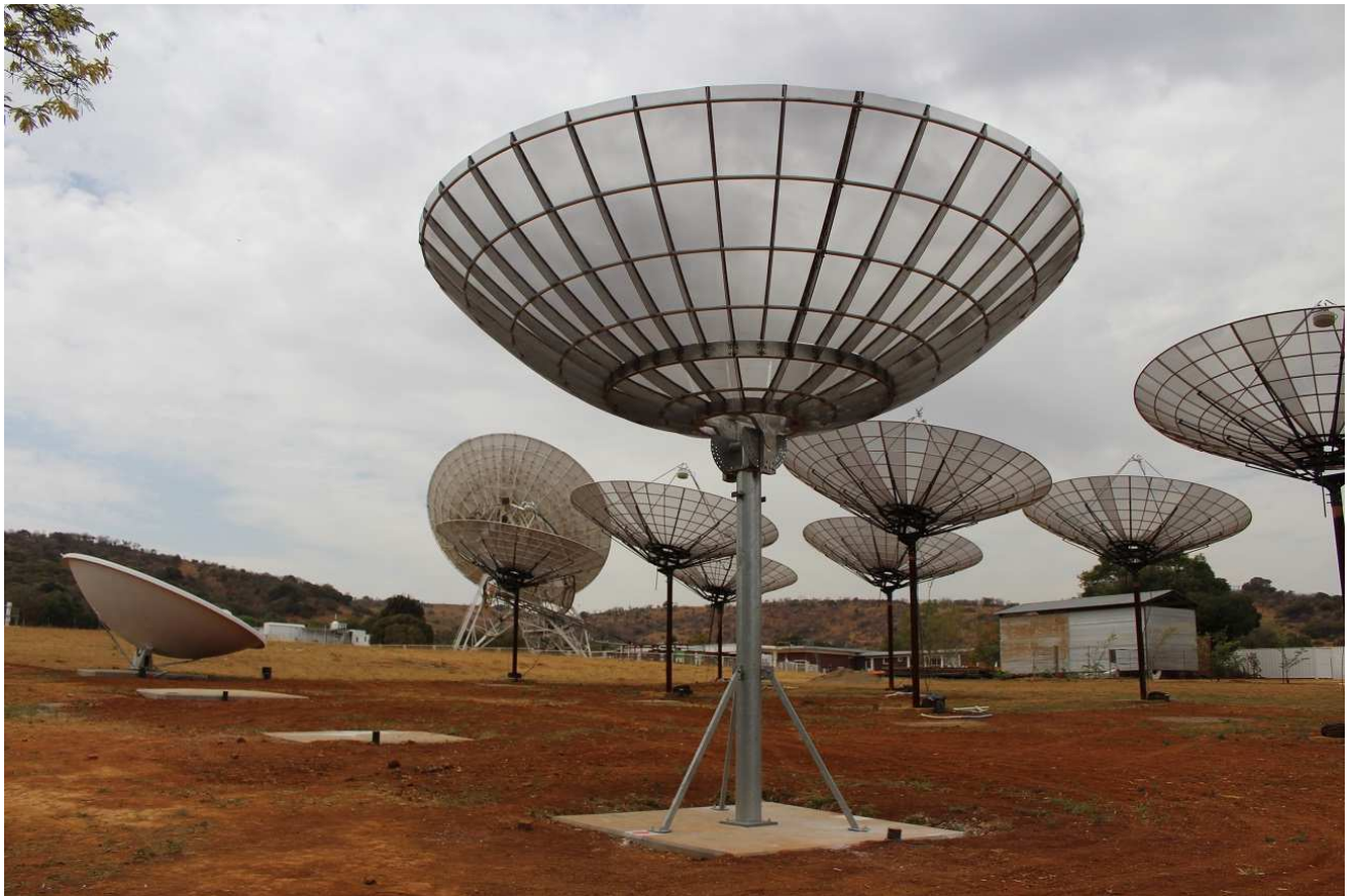
Fig 2. The 10-dish HIRAX prototype array in the foreground featuring the newly installed NJV Consulting/Rebcon dish at front and centre. The 26m dish at the SARA O Hartebeesthoek site is visible in the background.
