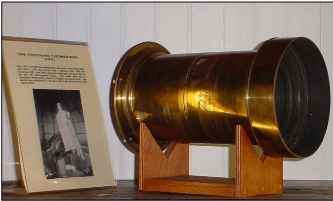
Fig 8. The Dallmeyer 6-inch diameter Rapid Rectilinear lens that was adopted by Gill for the Cape Photographic Durchmusterung. (Astronomical Museum, SAAO; photo: author).
