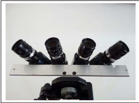
Fig 1. Low light video camera array used at Bredell. The cameras are Watec 904H cameras, set at f/1.2 , and with sensitivity of 0.0001 lux.
