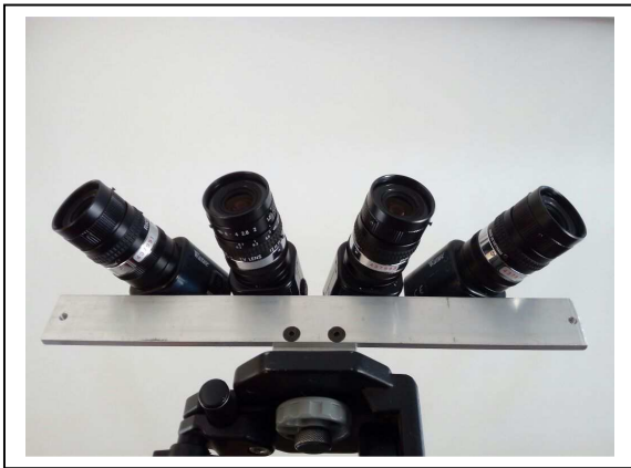
Fig 1. Low light video camera array used at Bredell. The cameras are Waterc 904H cameras, set at f/1.2 , and with sensitivity of 0.0001 lux.
