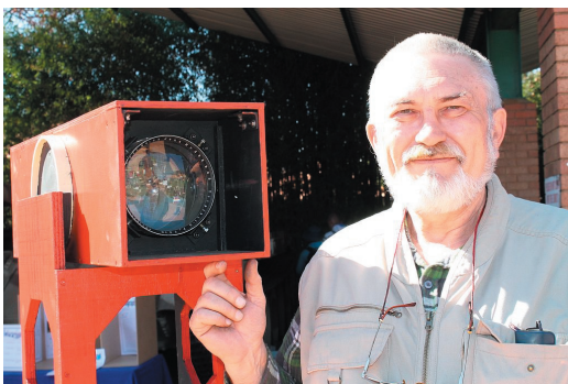
(above) Johan Smit revived this WWI vintage 700mm f/5 Zeiss aerial camera lens into a beautiful telescope.
