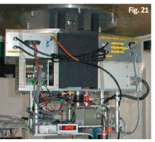
It was by far the most complicated camera that I had made. It was intended for use with a 512 x 512 pixel InSb array. Only a rather poor array, of "Engineering Grade" was available to me and even then, it turned out that the wiring diagram furnished with it was incorrect. Unfortunately the diagnosis of the problem only emerged after I retired. It caused the star images to be elongated in the declination direction.
