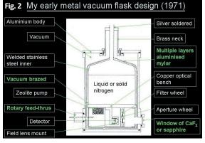
The Dewar I designed could hold liquid nitrogen for about 36 hours and so needed filling only once each day. The first one was in service for about 35 years and is now in the Astronomical Museum at SAAO. Another one is still in active use at Sutherland! Fig. 3 shows how the Dewar was mounted on a telescope as part of a photometer.
