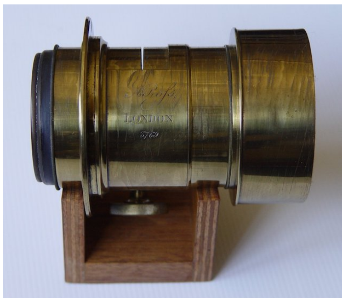
Fig 8: In 1882 a bright comet appeared and was photographed successfully by David Gill and a local photographer, Edward Haggard Allis, using this Ross lens (M049) of 2½ inches (64 cm) diameter and 11 inches (28cm) f.l. (Gill, 1913). It was strapped to the 6-inch Grubb telescope for tracking and guidance.
