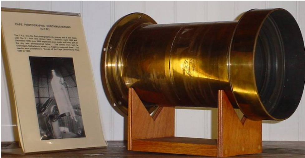
Fig 9: The Dallmeyer rapid Rectilinear Portrait lens Used for the Cape Photographic Durchmusterung or CPD catalogue.
