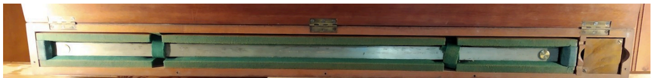
Fig 6: The upper item shown (M141a) is a standard “End Bar” of one yard.
