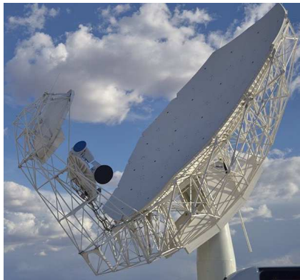
Fig 3. A single MeerKAT antenna. The configuration is an offset Gregorian. The radio signals bounce off the big dish onto the smaller one and then into the receiver just below the small one. Two receivers can be seen on the turntable. (Photo: S Burger, Engineering News).
