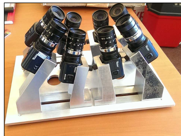
Fig 3. Watec 902H cameras mounted on aluminium mounts designed by Pieter Stronkhorst, and machined by Richard Moralo.
