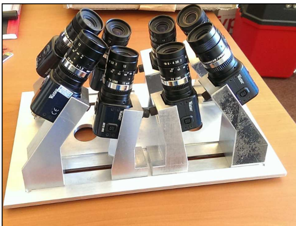
Fig 3. Wattec 902H cameras mounted on aluminium mounts designed by Pieter Stronkhorst, and machined by Richard Moralo.
