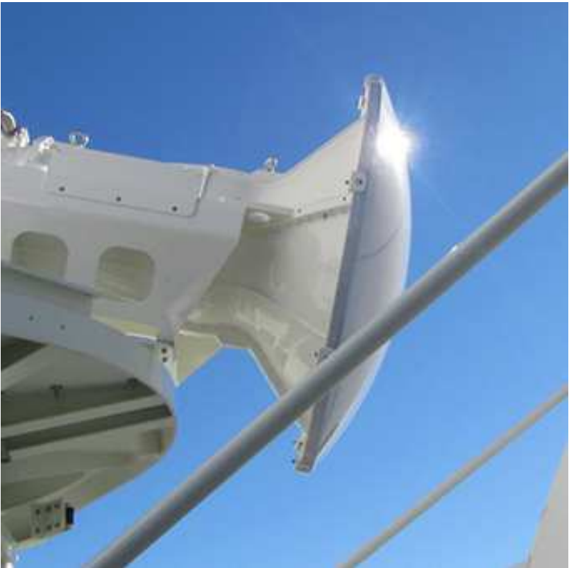
Fig 1: The Band 1 receiver’s protective cover reflects the desert Sun. To the right is the MeerKAT antenna’s secondary mirror. (Credit: SRAO)
