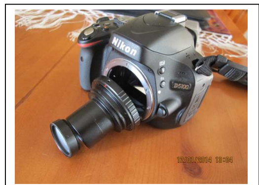
Fig 3. This shows the grating near the eyepiece with camera adaptor.
