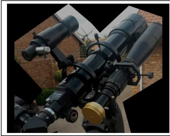
Fig 4. This shows the various instruments on the equatorial mounting. Left is the 80 mm refractor with the DSLR camera and grating fitted into the refractor tube where the eyepiece is currently (on the left), with the finder scope on the top. To the right is a 400 mm telephoto lens fitted with a ZWO130 CCD camera, used as a guide
