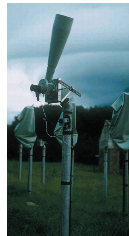
Apogee telescopes in Cape Town. The Apogee telescope was a great asset to the Moonwatch programme for several reasons, one of which was that it had a horizontal eyepiece which enabled long periods of uninterrupted observation. Image: Peter Smits
