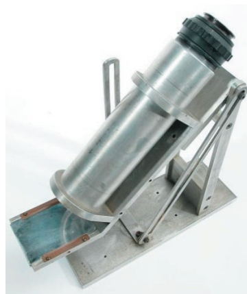
An example of an early Moonwatch telescope.
