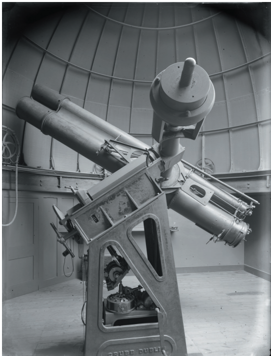
Fig. 3. The completed Astrographic telescope photographed around 1900. The large circular object inside the pier contained the governor for the clockwork motor.
