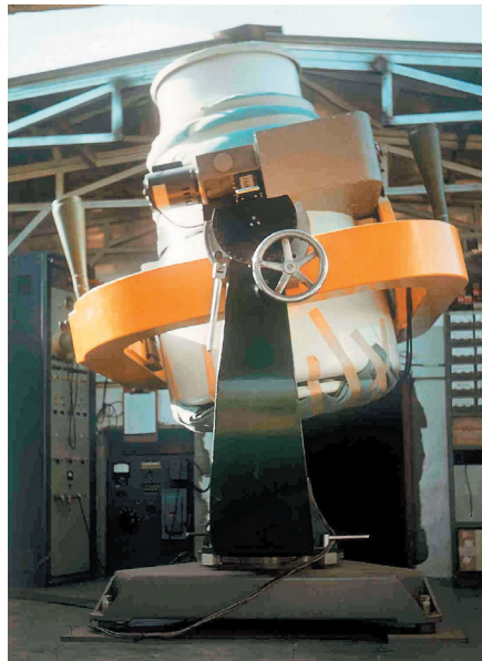
Baker-Nunn camera shortly after installation. Note the Norrman clock on the left hand side. Photo: Peter Smits
