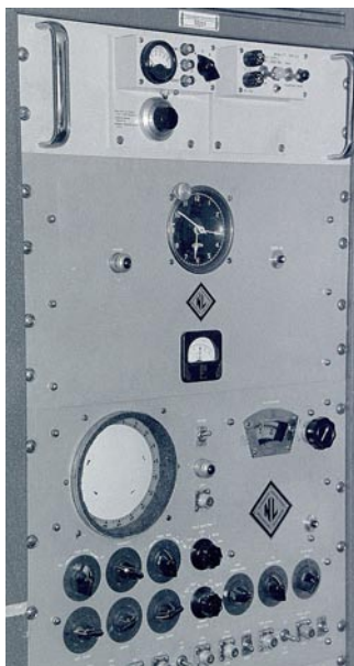
Norrman crystal clock. The cathode ray tube used to give a high resolution time display is obvious. Photo: Greg Roberts
