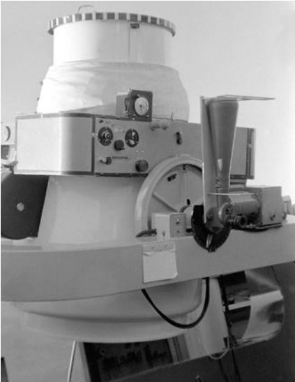
Baker-Nunn camera pointing to the zenith inside its triaxial mount with a 5-inch Apogee finder telescope mounted on the side. The top of camera has a thermal blanket wrapped around it. Photo: Greg Roberts
