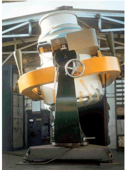
Baker-Nunn camera shortly after installation. Note the Norman clock on the left hand side. Photo: Peter Smits
