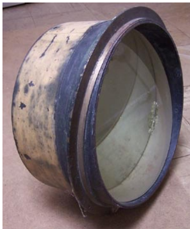
Fig. 6. The 12-inch diameter objective prism of 20° angle used by F. McClean with the Astrographic Telescope during his work on Oxygen in stars in 1897. This prism is owned today by the Norman Lockyer Observatory in Exeter, UK (Photo courtesy of M. Kaye).
