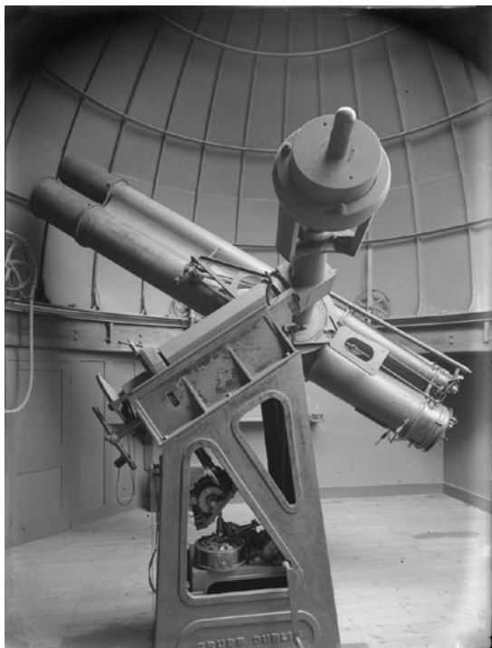
Fig. 3. The completed Astrographic telescope photographed around 1900. The large circular object inside the pier contained the governor for the clockwork motor.
