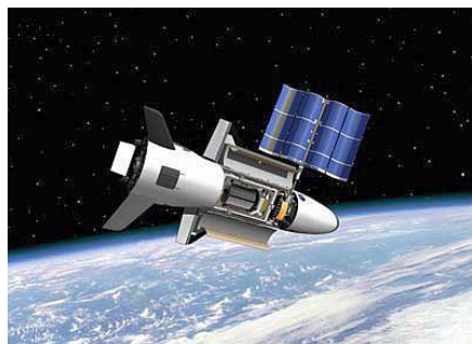
Artist's rendition of how the X-37B will deploy on orbit, including the solar panels used for electrical power. Image credit: Boeing
