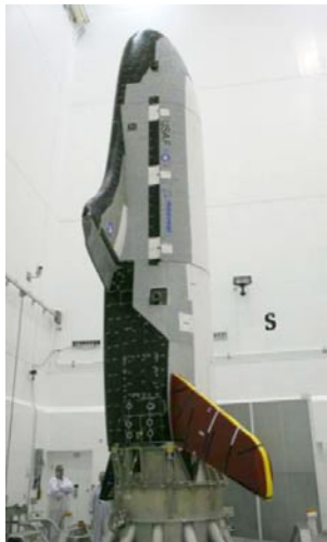
(left) The X-37 in a vertical attitude, the position in which it gets launched.
