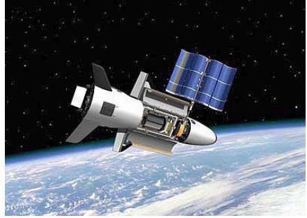
Artist's rendition of how the X-37B will deploy on orbit, including the solar panels used for electrical power. Image credit: Boeing
