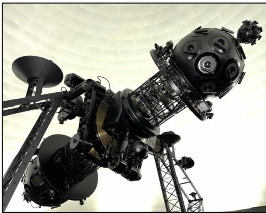
*Fig 8. MkIII planetarium projector manufactured by Carl Zeiss of Germany (Sourced by Kate Otten Architects).*
