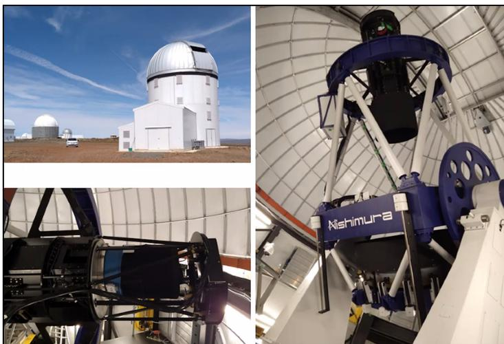
*Fig 2: Images of the PRIME telescope. The blue unit in the bottom left picture is the camera. Above it are the electronics and refrigeration units, themselves cooled to avoid air currents in the beam.*
