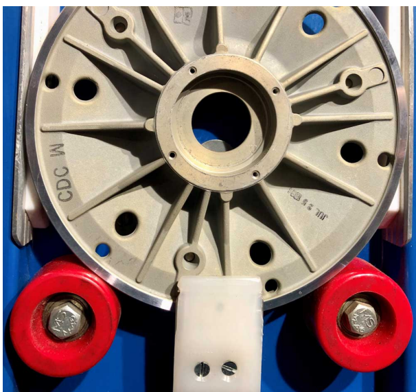
Fig 2a. Trunnion on rollers.
