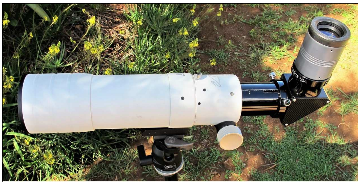
Image 3. The 2-inch 24 mm bisymmetrical on a WO Megrez apo.
