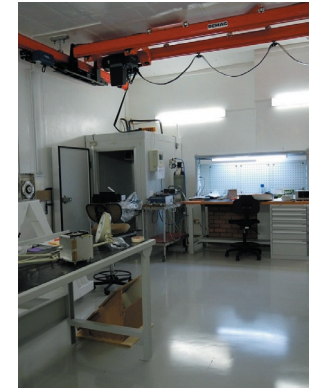
The Integration Room side of the optics lab during the removal of the old floor (left). This room now includes a new 1.6 ton overhead crane with an electric hoist, an environmental chamber for temperature-testing equipment and a large removable hatch in the wall shared with the Workshop to allow large instruments to be moved in and out.
