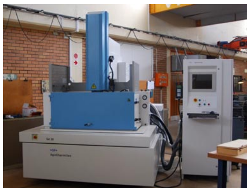
(left) The CNC Spark Eroder. The blue turret holds the tool electrode and moves it up and down (in the Z-direction). The blue door seals the work volume that gets filled with dielectric fluid and the part gets clamped to
