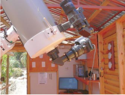
Fig. 5: Camera mounted for afocal photography.
