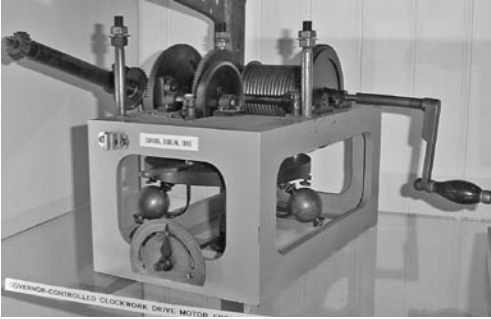
The original Grubb governor-regulated, weight-driven clockwork motor of the 6-inch telescope (above). Chemical apparatus include a mortar and pestle (top-right) and electrometer valves (right).
