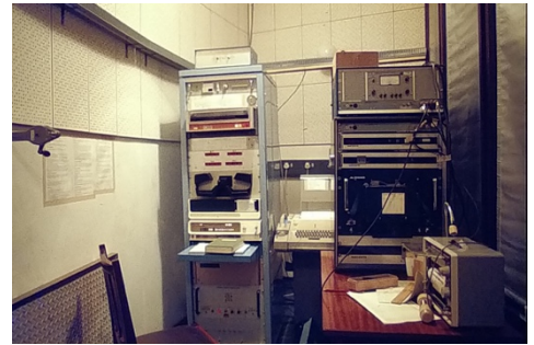
Fig 2: The first warm room in the 74-inch. On the left is the Nova computer with a 2.5MB(!) disc drive, a paper tape reader and a Teletype terminal. On the right is the infrared recording equipment with paper tape output and a chart recorder.
