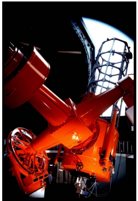
Fig 4: The 74-inch in its orange coat! Attached at Cassegrain is an infrared photometer with the ISEC camera in blue. The F/50 infrared chopping secondary, only 18cms in diameter, is in place (Photo: Cibachrome by RM Catchpole).
