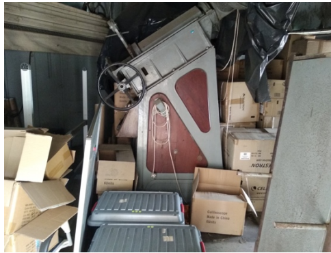
Fig 2: The telescope in its original form. Originally constructed for photographing the Cape Zone (between declinations -40^{\circ} and -52^{\circ} ) of the international Carte du Ciel project, it has had an interesting and varied history.
