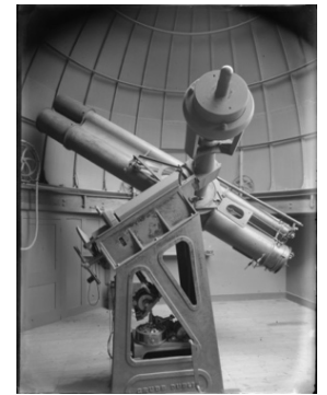
Fig 2: The telescope in its original form. Originally constructed for photographing the Cape Zone (between declinations -40^{\circ} and -52^{\circ} ) of the international Carte du Ciel project, it has had an interesting and varied history.
