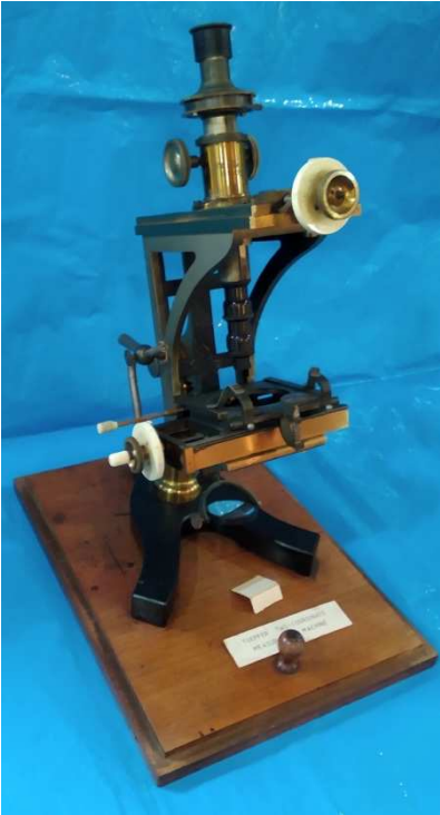
Fig 5. Zeiss blink comparator. Probably adapted from a viewer for stereoscopic plate pairs (SAAO Museum Cat. # M155).
