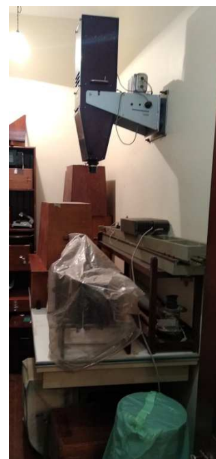
Fig 25. The Demac machine. It consisted of a projector mounted on the wall and a digitizing table (seen here cluttered with other items). It is in a small room now used as the Museum Store in the McClean dome (SAAO Museum Cat. # M181).
