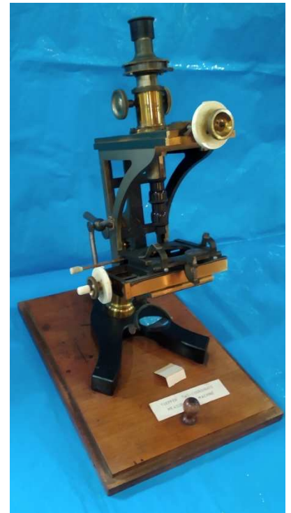
Fig 4. Toepfer measuring microscope in SAAO Museum (Cat. # M149).
