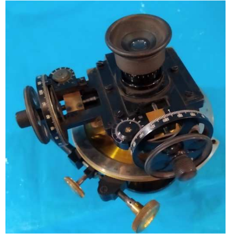
Fig 7. Stereoscopic attachment for Zeiss Blink. This replaces the blink part (SAAO Museum Cat. # M064). In own wooden box.
