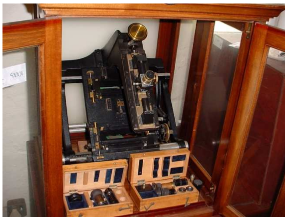
Fig 15. Hartmann spectro-comparator (SAAO Museum Cat. # M162).
