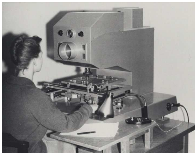
Fig 21. Sartorius Iris photometer (photo: SAAO P4282)
