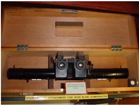
Fig 7. Stereoscopic attachment for Zeiss Blink. This replaces the blink part (SAAO Museum Cat. # M064). In own wooden box.
