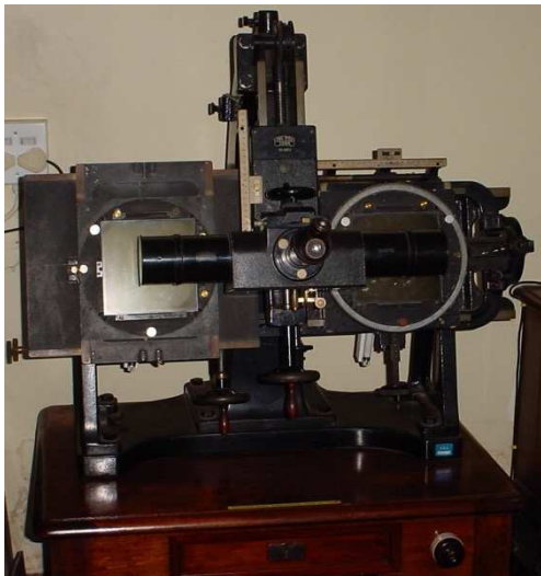
Fig 5. Zeiss blink comparator. Probably adapted from a viewer for stereoscopic plate pairs (SAAO Museum Cat. # M155).
