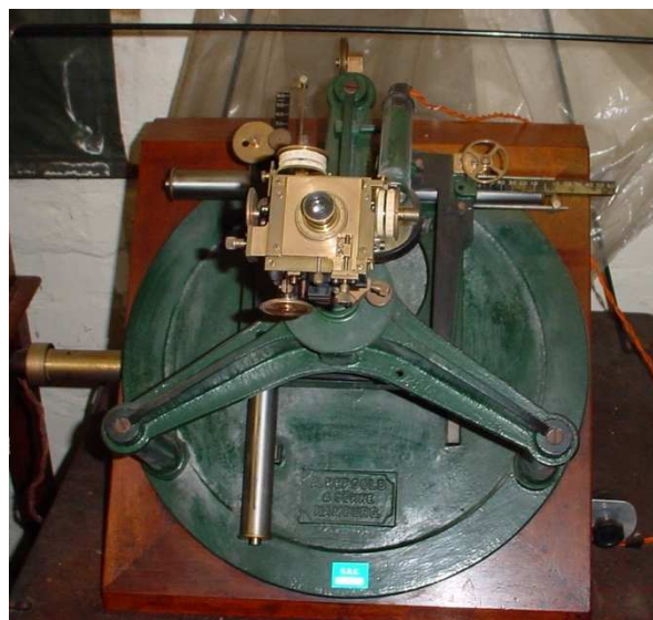
Fig 2. The Gill measuring machine, built by Repsold of Hamburg. Two were constructed (SAAO Museum Cat. # M178, # M179).
