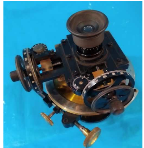
Fig 7. Stereoscopic attachment for Zeiss Blink. This replaces the blink part (SAAO Museum Cat. # M064). In own wooden box.
