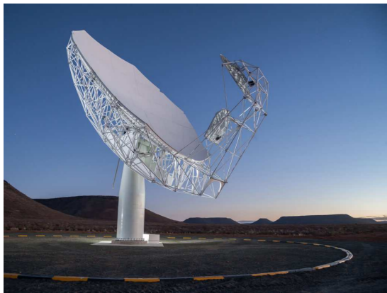
Fig 4. A single MeerkAT antenna. The radio signals bounce off the big dish onto the smaller one at right and then into the receiver just below the small one (Photo: SAAO).
