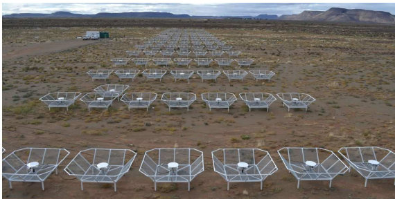
Fig 15. Paper was a relatively simple precursor array located on the SKA site with the same aim as HERA. It was too small and insensitive to achieve the desired aim and has now been superseded (Photo: University of California Berkeley Astronomy Website).
