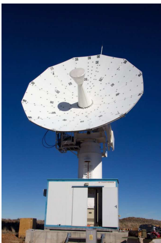
Fig 11. The C-bass antenna at Klerefontein near Carnarvon. It has a diameter of 7.6m and was donated by Telkom.
