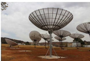
Fig 13. Prototype antennas for HIRAX under test at Hartebeesthoek (Photo credit: SARA0).
