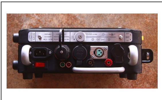
Fig. 11 Front panel: Left to right: 220VAC mains input (switch below); USB charging port (charging status lights below); Cigarette lighter, XLR & Hella connections for 12VDC out (Binder posts for external battery below); internal/external battery selector switch hidden behind protective handle.
