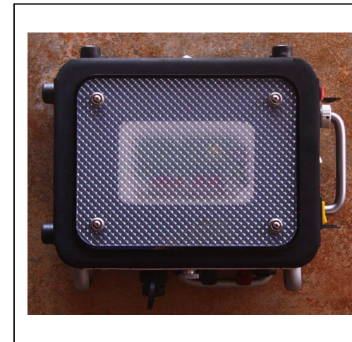
Fig. 12: LED lamps. These are covered with a prismatic diffusing filter. The greenish zone has four high-intensity white LEDs. Below those can be seen the red of the night-vision friendly dimmable red LEDs. To the top right is the red switch to control the red LEDs, below which is a silver knob to control the brightness. At bottom right is a yellow rocker switch to control the white LEDs. This has three positions: latching On, Off, and momentary On positions.
