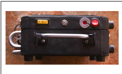
Fig. 13: Top view. This is conveniently arranged to control the white light whilst walking (either left- or right-handed). Also visible is the view side of the battery selector switch, nestled in the protective handle.
