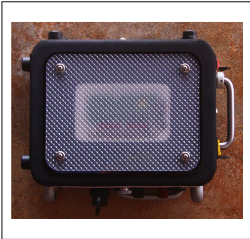
Fig. 12: LED lamps. These are covered with a prismatic diffusing filter. The greenish zone has four high-intensity white LEDs. Below those can be seen the red of the night-vision friendly dimmable red LEDs. To the top right is the red switch to control the red LEDs, below which is a silver knob to control the brightness. At bottom right is a yellow rocker switch to control the white LEDs. This has three positions: latching On,
