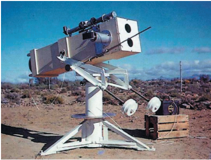
Fig. 17: One of the Danjon telescopes, taken in 1962 during the last stages of site testing, here fitted with a mask to simulate a double beam telescope for measuring image motion. Credit ESO, D Beintema
