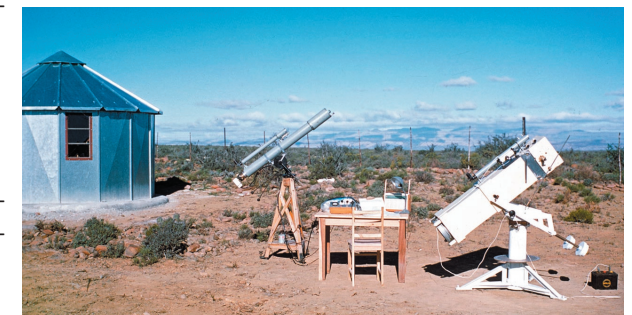
Fig. 4: A typical ESO site testing station in 1961. On the right is the 25-cm Danjou-telescope, used to measure the seeing, while the little photometer on the left is monitoring the transparency of the atmosphere. Credit: ESO, W Schlosser
