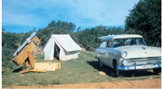
Fig. 5: This picture shows the observing post on the Rooiberg hill near Cillitzdorp in the southern Karroo, with a Danjon telescope equipped with a Walraven refractor-photometer. The car is one of the two Ford Range Wagons used by the parties. The picture was taken by one of the principal participants of these site tests, J Dommanget. Credit: ESO, J Dommanget
