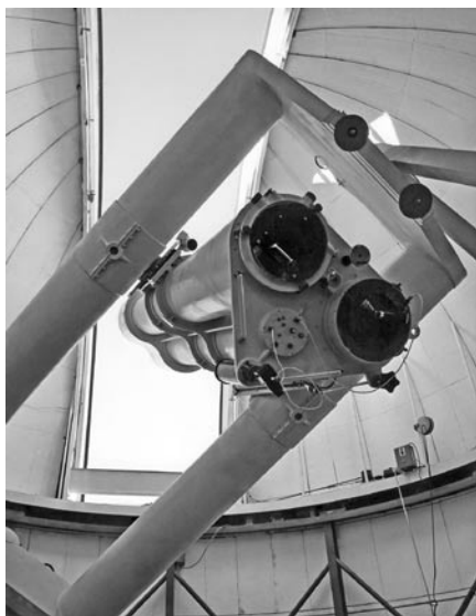
Fig. 14: (below) The GPO (Grand Prisme Objectif Telescope), here at La Silla in 1968, first operated in Zeekoegat, South Africa from 1961 to 1966. The GPO is a copy of a telescope installed at the Observatoire de Haute Provence in France. One half of the telescope is a 40-centimetre objective prism for obtaining the spectra of many objects at the same time. The other telescope is for guiding. Credit: ESO
