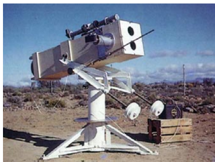
Fig. 17: One of the Danjon telescopes, taken in 1962 during the last stages of site testing, here fitted with a mask to simulate a double beam telescope for measuring image motion. Credit ESO, D Beintema
