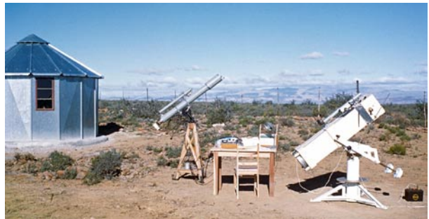
Fig. 4: A typical ESO site testing station in 1961. On the right is the 25-cm Danjou-telescope, used to measure the seeing, while the little photometer on the left is monitoring the transparency of the atmosphere. Credit: ESO, W Schlosser
