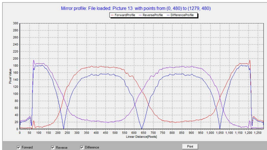
Fig 5 - Pixel intensity profiles, forward, reverse and difference. Only left hand null need be read.
