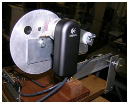
Figure 11 (below) - Rear of tester showing CCD webcam and adjusting and panning arms.
