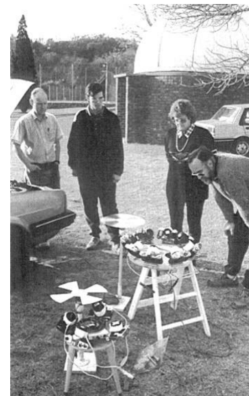
joined us having brought several camera platforms with rotating segmented disks used to determine meteor velocity and duration (Figure 11).
