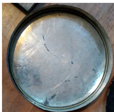
Fig 7. (left): The lower part of the tinned box that surrounded the mirror. The brass rod around the inner edge can be seen.
