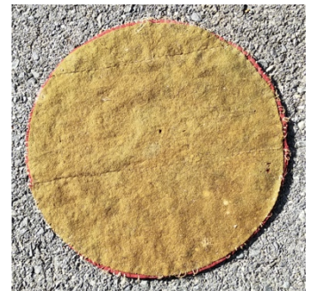
Fig 10. Pad, consisting of 4 layers of blanketing material sewn together, found behind mirror.
