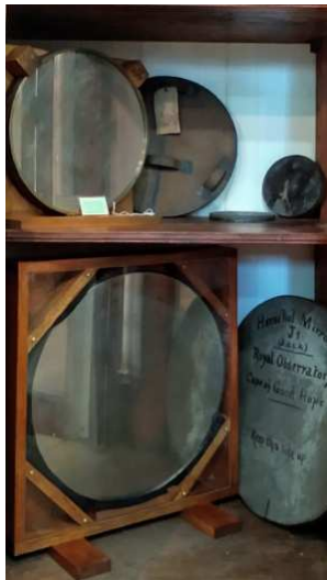
Fig 11. A new box with a Plexiglass cover, to display the 20-foot mirror in a vertical position, has been constructed and is shown in the lower part of the figure together with the lid of the mirror tin. Above it is a 14-foot mirror and lid, constructed by William Herschel in 1810; (See Warner, B., MNASSA 1987, 46 , 158); also a smaller concave speculum mirror of about 15 cm diameter of unknown provenance.
