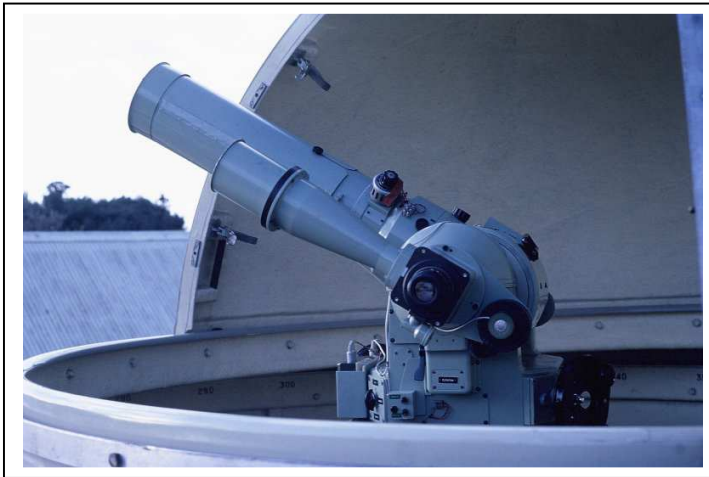
Fig 1. The Cape Kinetheodolite (photo: G. Roberts).
