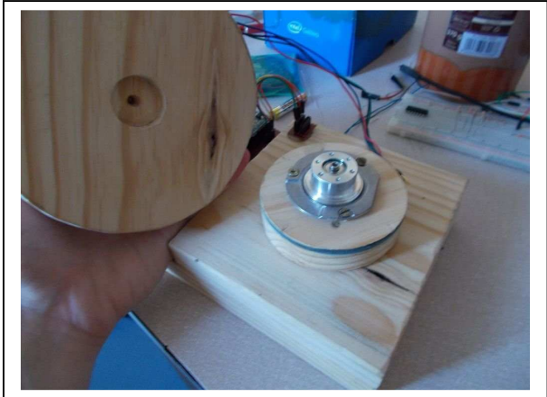
Fig. 3 (right) Showing the large and small wheels. Note the groove to carry the precision drive belt (knotted elastic band!)
